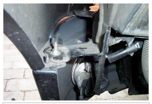
Still sitting on the floor; remove the M6 nuts which are holding the bumper edges on it's place.
