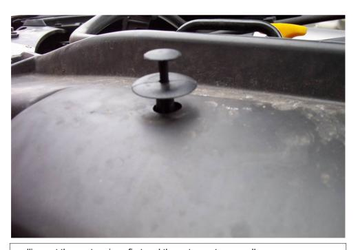
pulling out the centre piece first and the outer parts secondly.
