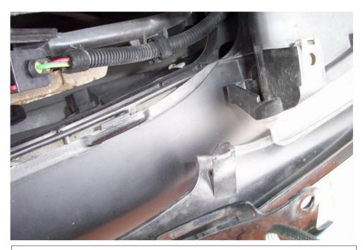
The remaining clips holding this piece to the headlights are sitting low in the corners. Push them one at the time downwards and release it from the headlight unit.
