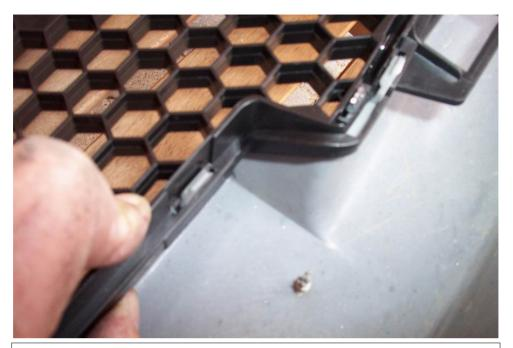
Support the bumper from the underside and put the new grill into place.
