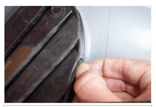
If one wants to take out the grill, put the bumper down on the grass (or something else soft and non-scratching) with the backside up. The grill is simply clipped on the bumper by means of several retraining clips, moulded in the bumper. It's fairly easy to take it off.
