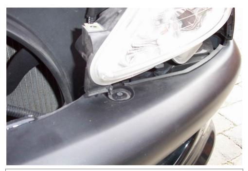
Now the M6 Torx30 bolts under the headlights have to be taken out. This is possible without removing the headlight units...
