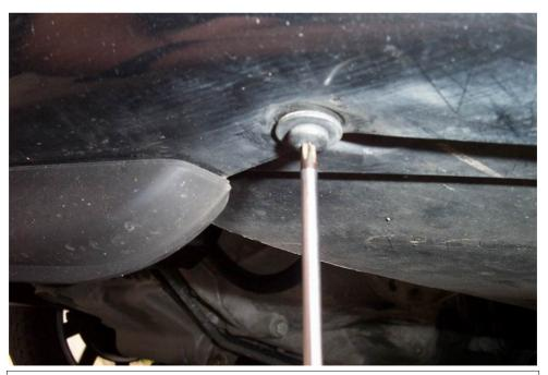
Crawl under the car and remove the two Torx20 parkers, positioned left and right of the spoiler...
