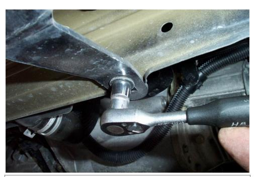
We're almost there: remove at the underside of the bumper the two M6x20 bolts, which are connecting the bumper with the steel transverse chassis bar...
