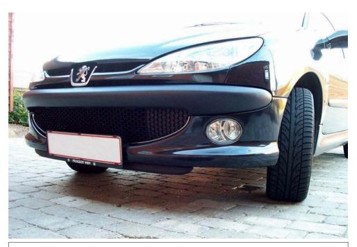
To put the bumper back, simply go in reverse order, minding the paint and noting that the front inner wings have to be slid back **under** the rear half of the inner wing. Keep also the markings in mind when you put the various nuts, bolts and parkers back, so all the items you removed will be bolted tight in the same position as they were. Then it looks like this...
