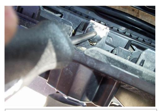
Loosen the M6 Torx30 bolt located bang in the middle, just behind the lion.
