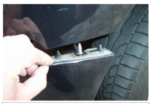
...pull the bumper edges down, out of the arches and call a mate and ask him to hold the bumper!
