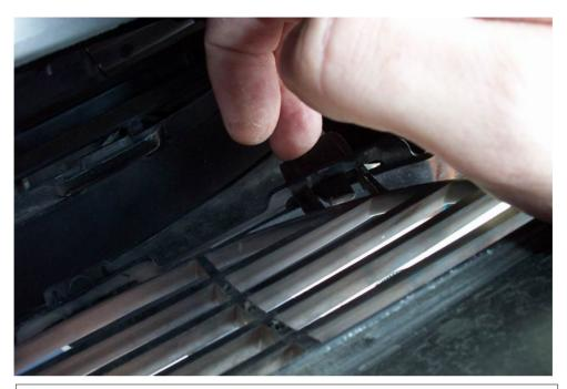
Grab down behind the grill and loosen it by simply squeezing the six clips one by one...
