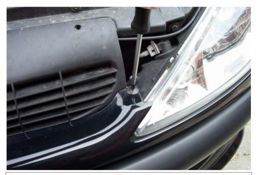
Remove the M6 Torx30 bolts, situated on the two ends of the upper grill.
