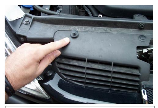
Remove the four mushroom clips (holding the plastic grill to the car) by...ae second one three ribs to the right of the filler hole, in the middle between the two longitude ribs
