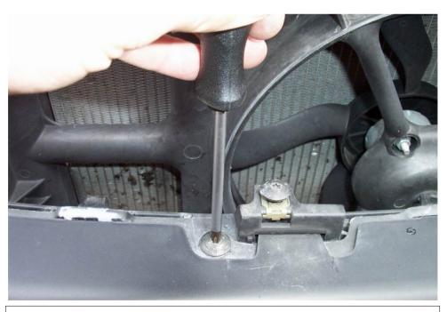
The last thing holding the bumper on its place is a Torx20x30 bolt positioned in the middle of the bumper, in-between the head lights, just left from the Torx20 bolt you loosened in step 9
