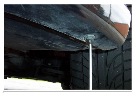
...and remove the remaining two Torx20 parkers left and right around the corner, close to the front wheels.
